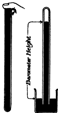
FIG. 73.—This type of barometer may be easily and quickly made.
